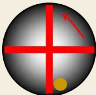
Tower mill - grinding energy imparted through the stirrer
